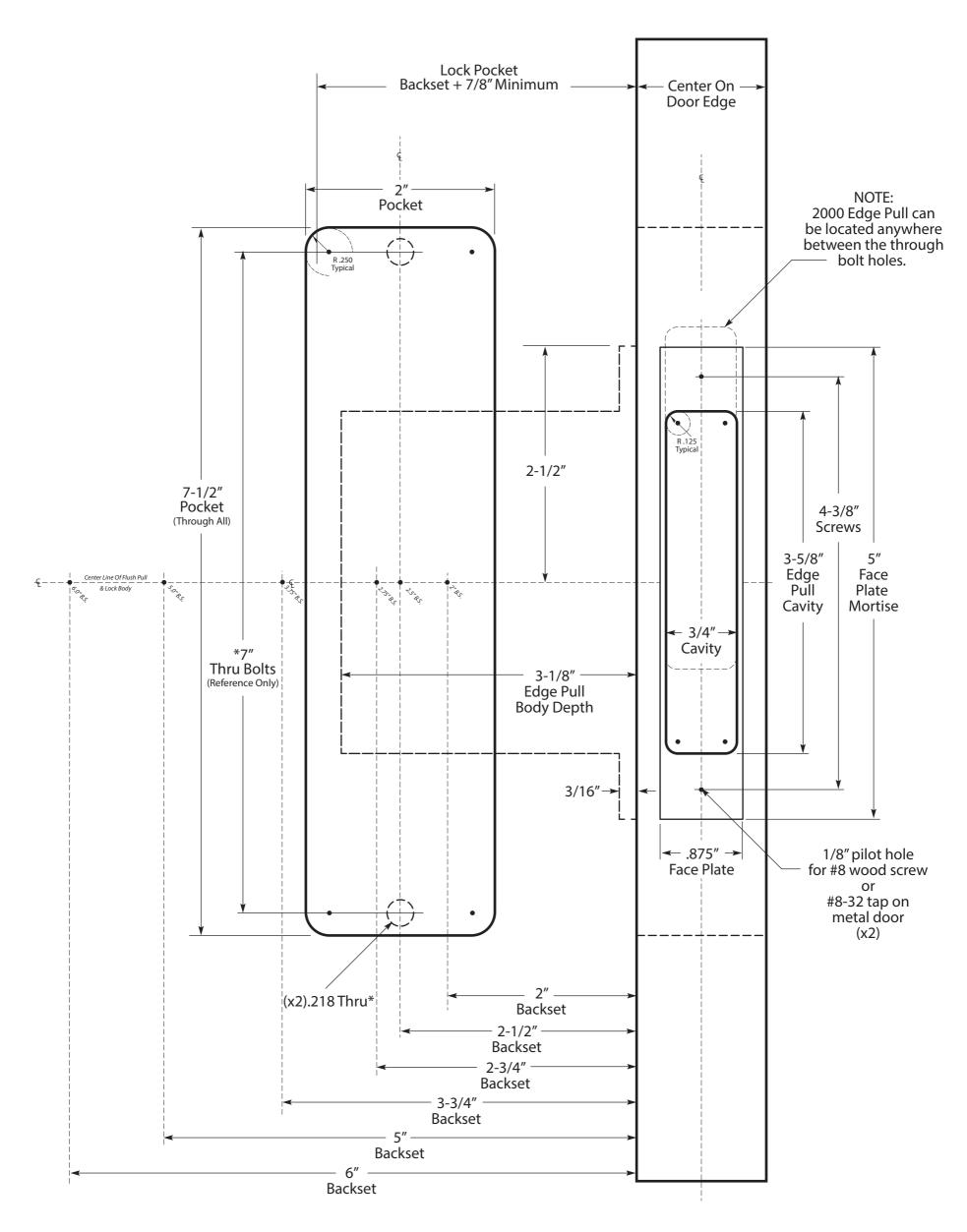
Backset is determined by door manufacturer or the end user. The Edge Pull has no bearing on this measurment.
